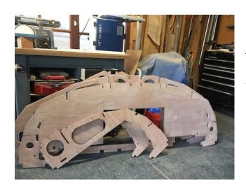
The boat is of Okoume plywood/ epoxy construction with Eucalyptus trim. Chase Small Craft in Maine provided the cnc cut plywood and milled timber.
