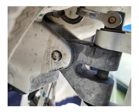
During a calm interlude, Mike and Alan went forward and noticed a broken cotter key on deck and that a pin holding the mast toggle to the boom was working its way free. For the remainder of the voyage, each watch would inspect the pin and pound it back in to position if required.
