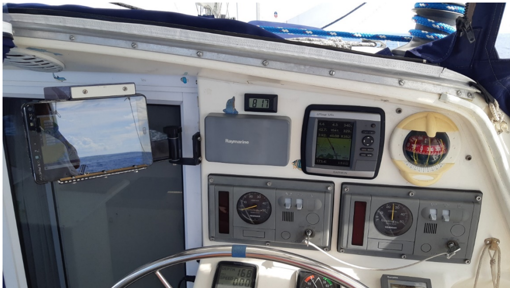
Soggy Paws helm station with Garmin 526S chart plotter on right and Asus tablet on the left
